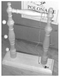
**Tensioned lazy kate** - Screw two eyescrews into the predrilled holes on the base. Insert the ends of the short piece (handle) into the predrilled holes at the top of the two long posts. Now press the bottom of the two longer posts into the base ensuring that the small hole in the handle is at the same end as the two eye screws. Glue base if you want to make a secure, permanent unit. Attach the Lazy
