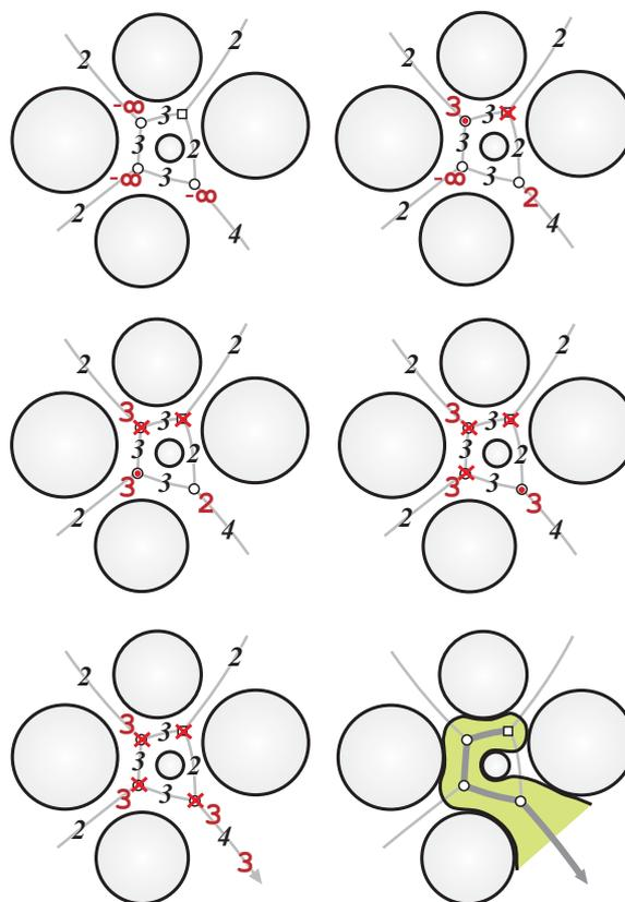
**Figure 5. Example of Dijkstra algorithm progress.**
